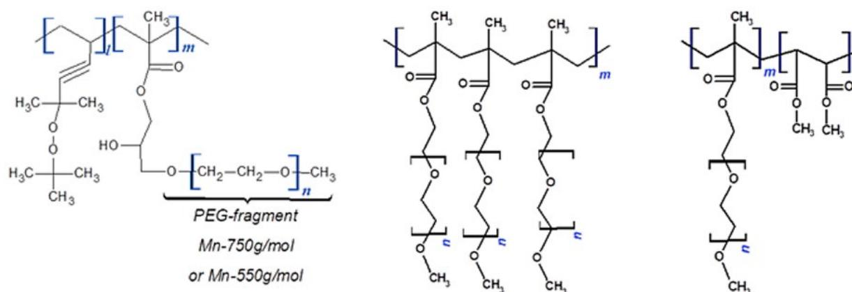
**Fig. 2.** Structure of PCs: A — poly(VEP-co-GMA)-graft-mPEG ( $k = 1.4$  % mol,  $l = 98.6$  % mol,  $M_n = 240$  kDa); B — poly(PEGMA) ( $k = 99.2$  % mol, [IPB-fragment] = 0.8 % mol,  $M_n = 55$  kDa); C — poly(PEGMA-co-DMM) ( $k = 87.0$  % mol,  $l = 13.0$  % mol,  $M_n = 47$  kDa).
